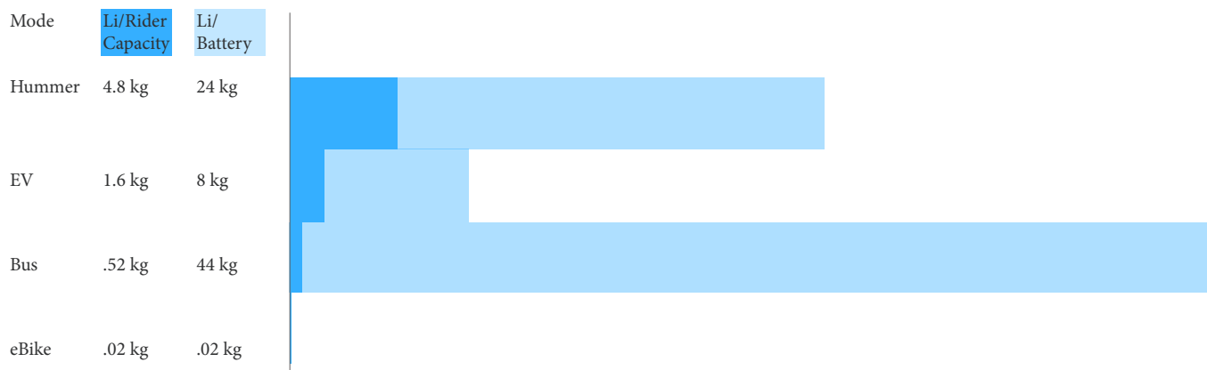
Figure 4. Comparative chart of e-Hummer, EV, e-bus, and e-bike lithium intensities.
